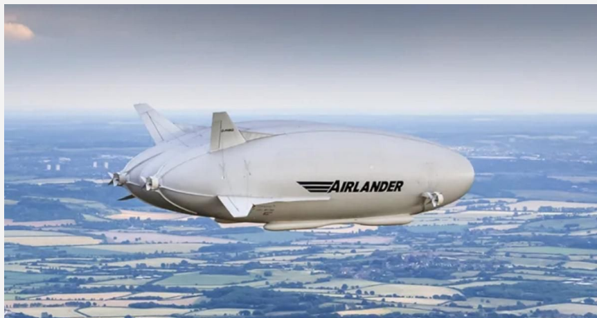
The Airlander (the Flying Bum) is a British helium airship with a unique design that uses both aerostatic and aerodynamic lift to fly
