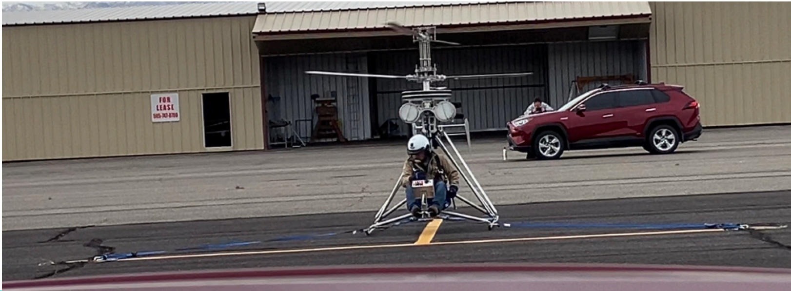
John George conducting tethered flight testing of his SCH-2A at Espanola Airport.
