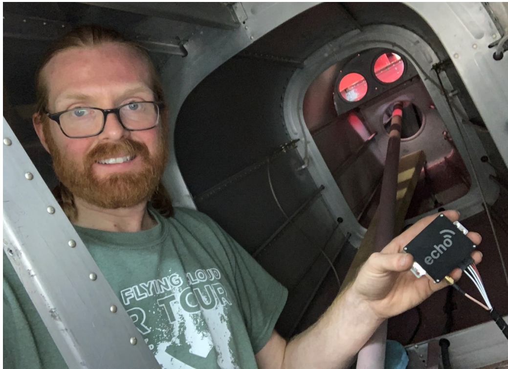
Figure 5: Your presenter, installing an ADS-B transceiver into an RV-7A kitplane in 2019. Credit: Keith Tschohl
