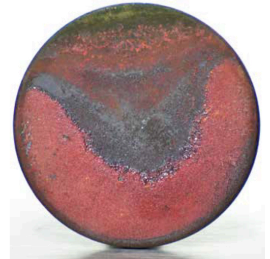
Top: Borecope picture of an exhaust valve stem with heavy deposits that can lead to a stuck valve. Bottom: An exhaust valve destined for failure with the dead green crescent.
