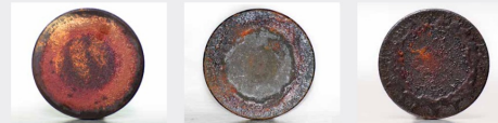
Don't be alarmed by the bright color, or deposits around the edges. The symmetrical pattern shows this valve is just fine. A symmetrical, circular pattern shows a healthy valve. Red and orange deposits are harmless. Thick lead deposits from an overly rich mixture give this healthy valve the appearance of an overcooked pizza.
