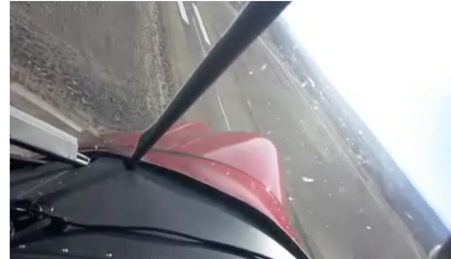
A turn back to the runway after an engine failure on takeoff will require aggressive maneuvering near the ground.
