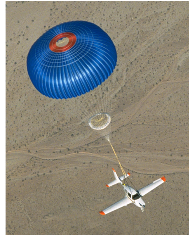
Effective ballistic recovery systems exist today for light aircraft and have proven to be life savers in an emergency over and over again.
