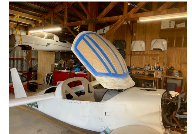
The rebuilt canopy is back on it's hinges on the Dragonfly. Skip is in the process of doing the final fitting work.
