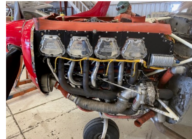
An eight cylinder, twin turbocharged, 400+hp Lycoming TSIO-720 on a Piper Comanche in a hangar down at Double Eagle Airport.
