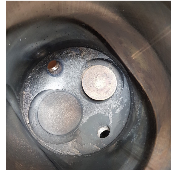
The exhaust valve on this Lycoming is stuck open.
