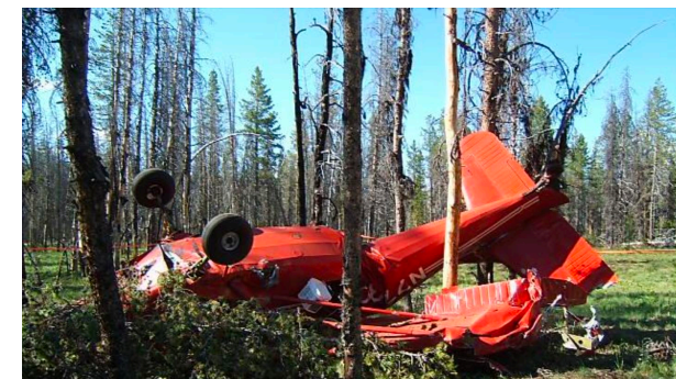
This wrecked Stinson 108-3 is a result of the pilot trying to takeoff with a density altitude equal to his service ceiling.
