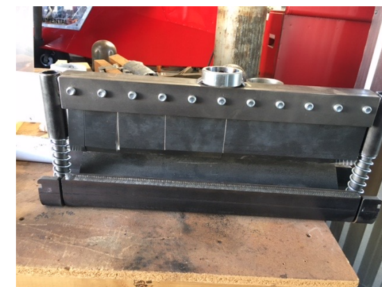
The fixture in the 40 ton press (top), is designed to make large radius bend in titanium. Press brake (bottom), has a punch with a small radius that can create stress concentration in a part.
