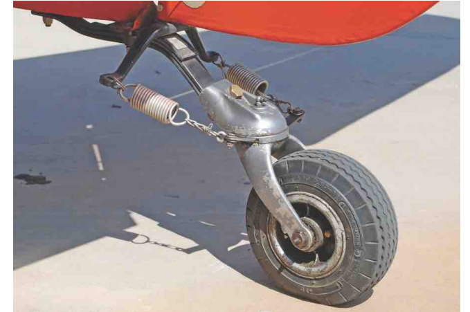
Scott tailwheel assembly with built in shimmy damper. Courtesy of Dave Prizio, Kitplanes.
