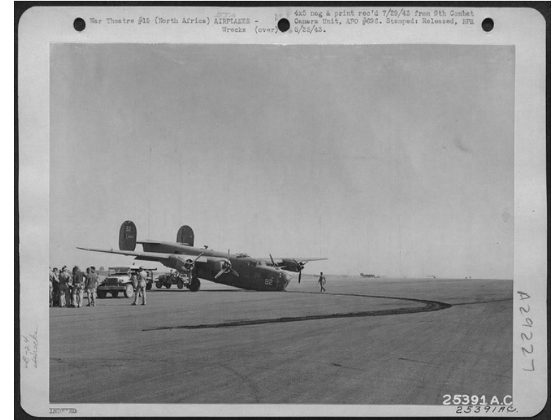
A B-24 Liberator, shown after suffering a nose wheel failure at a base in North Africa. Nose wheel shimmy was a serious enough problem that they often carried a replacement nose gear with them on cross country flights.
