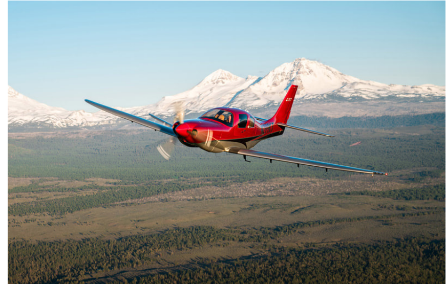
RDD Enterprises LX-7 has improved upon the stall characteristics of the Lancair IV-P and added a whole aircraft parachute system.
